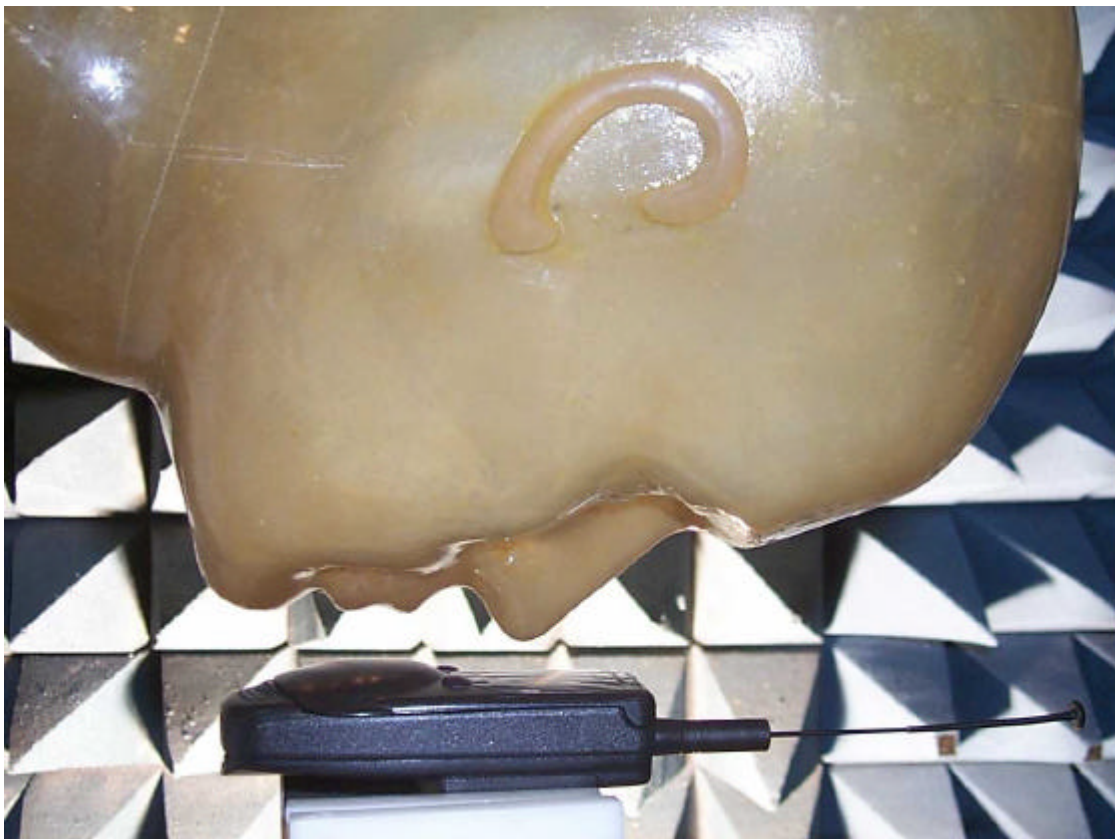
Figure 11. Diagram showing typical alignment of radio held to face.
