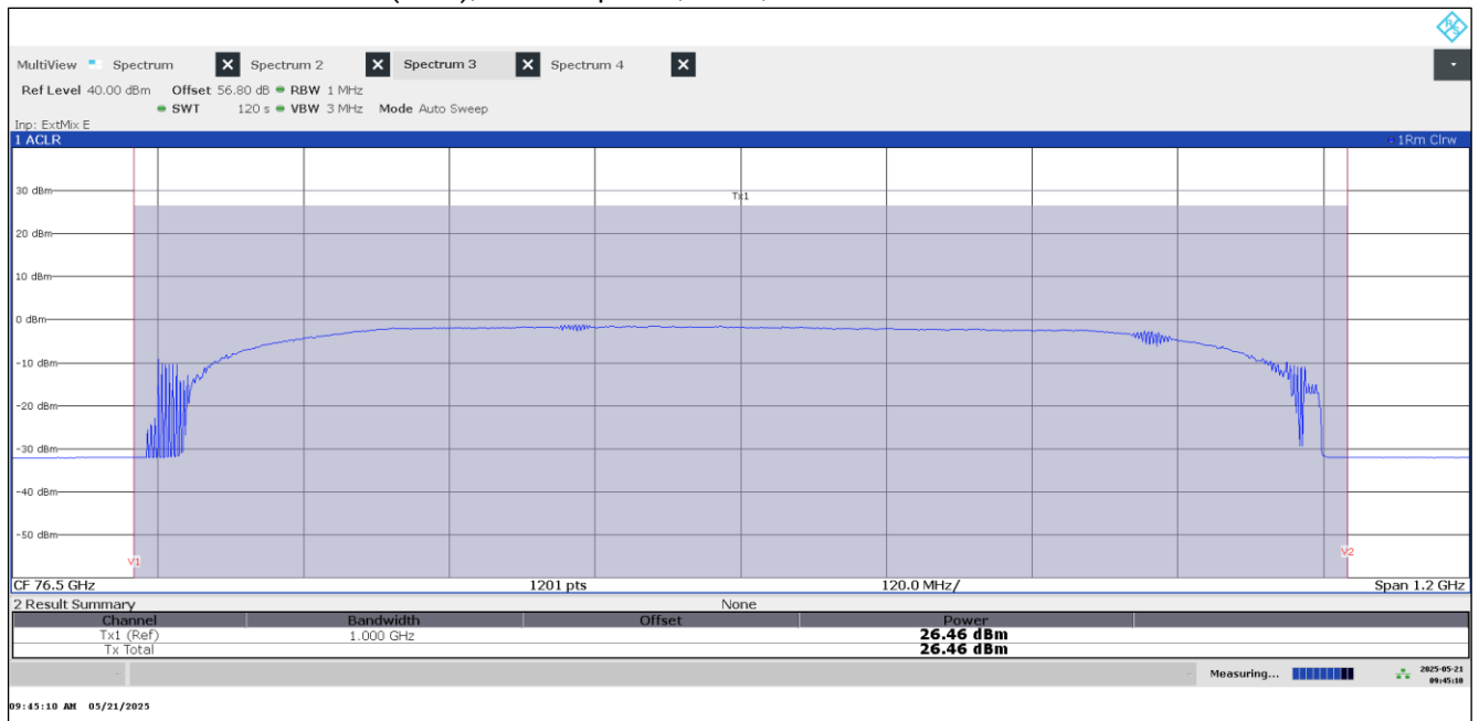
Plot 3: Radiated Mean Power (EIRP), Channel power, EUT1, Mode 02
