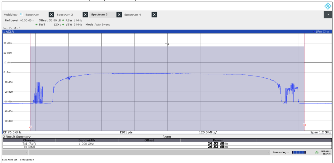
Plot 7: Radiated Mean Power (EIRP), Channel power, EUT1, Mode 04
