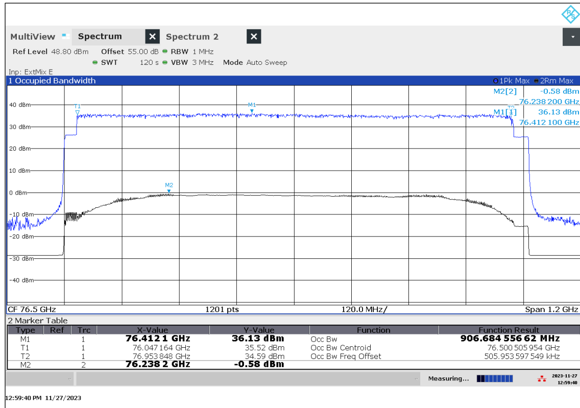
Plot 5: OBW, Mode 09, T_{\min} / V_{\min-\max}
