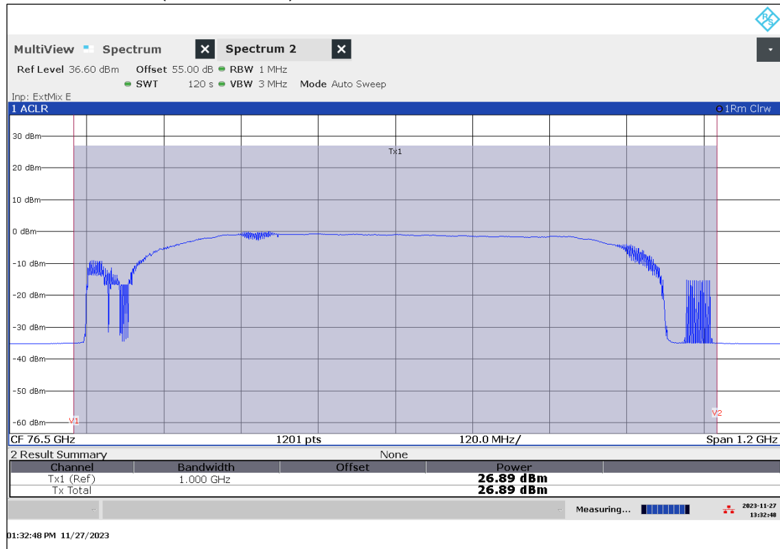
Plot 38: EIRP Mean Power (Channel Power), Mode 21, RMS detector, T_{\min} / V_{\min-\max}
