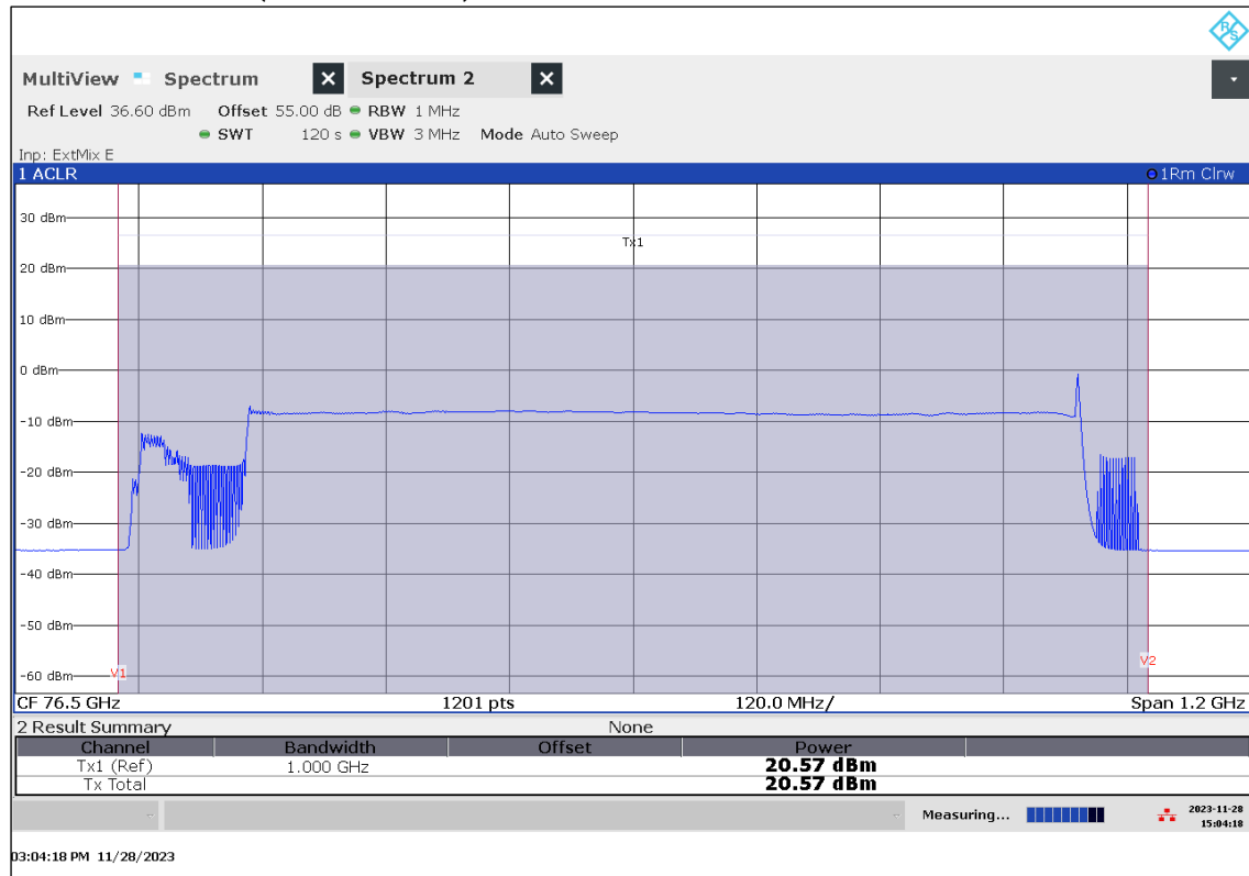
Plot 54: EIRP Mean Power (Channel Power), Mode 80, RMS detector, T_{\max} / V_{\min-\max}
