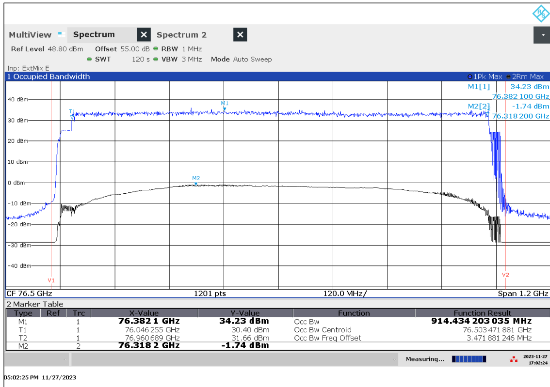
Plot 80: Mode 09, OBW, 10 °C / V_{\min-max}
