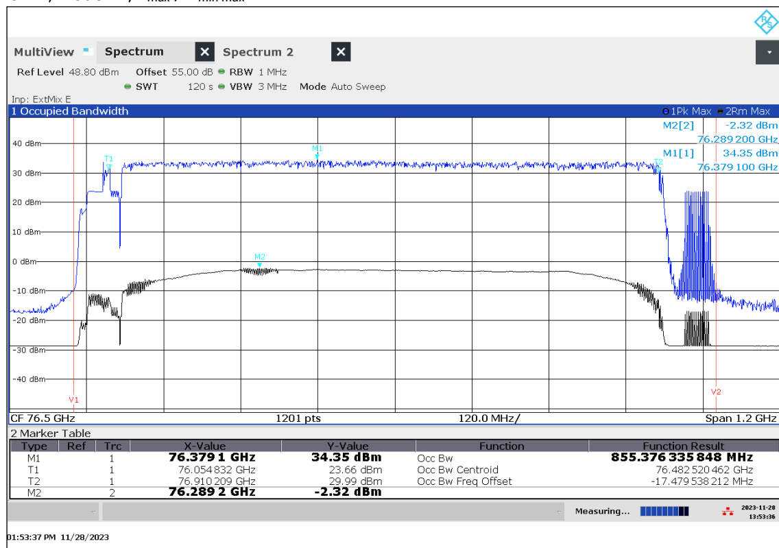
Plot 12: OBW, Mode 21, T_{\max} / V_{\min-\max}
