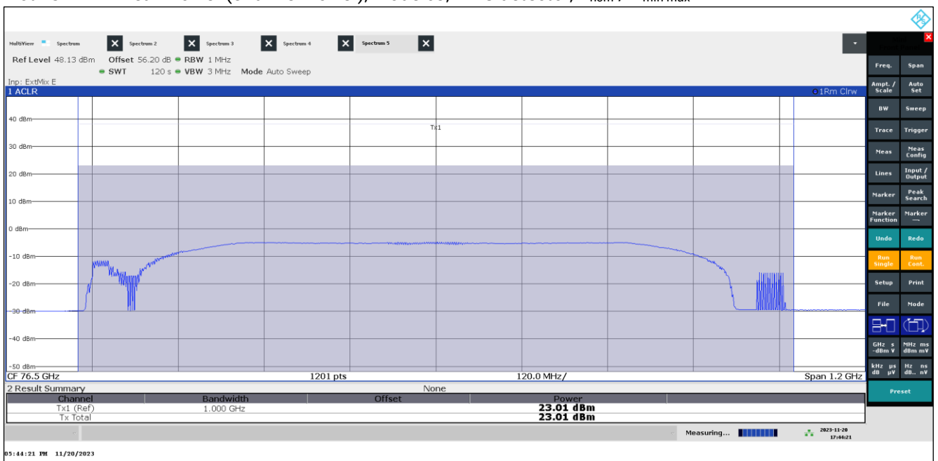
Plot 49: EIRP Mean Power (Channel Power), Mode 63, RMS detector, T_{\text{nom}} / V_{\min-\max}
