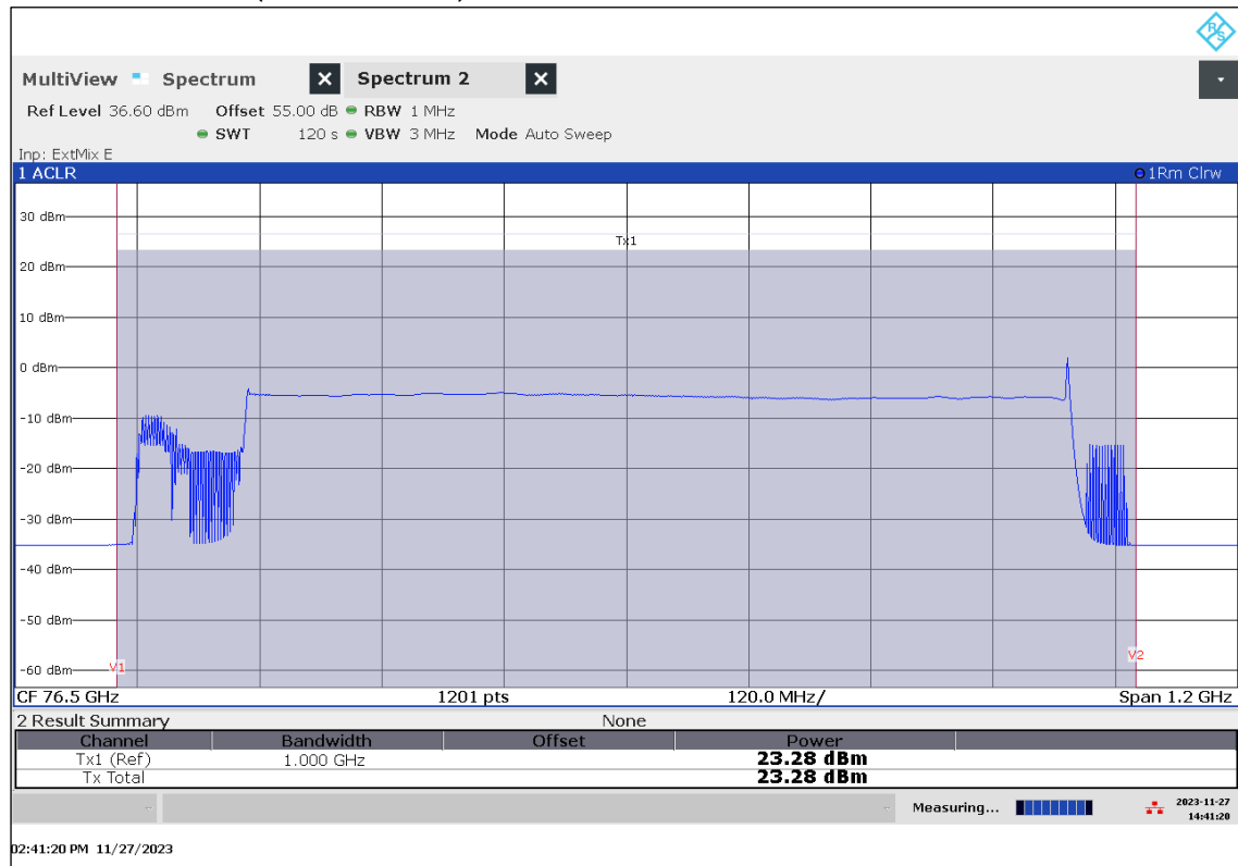
Plot 53: EIRP Mean Power (Channel Power), Mode 80, RMS detector, T_{\text{min}} / V_{\text{min-max}}
