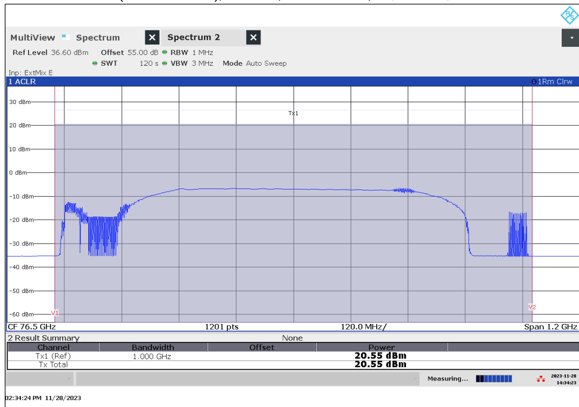
Plot 48: EIRP Mean Power (Channel Power), Mode 51, RMS detector, T_{\max} / V_{\min-\max}
