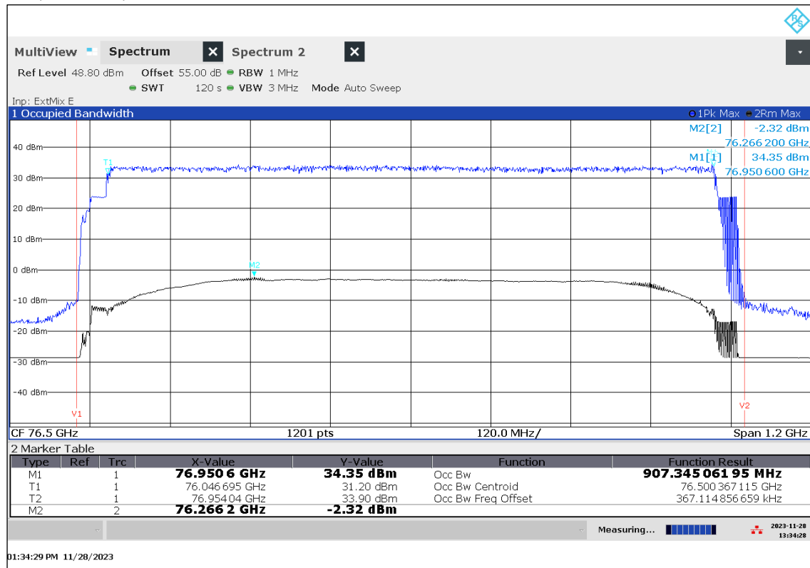
Plot 6: OBW, Mode 09, T_{\max} / V_{\min-\max}
