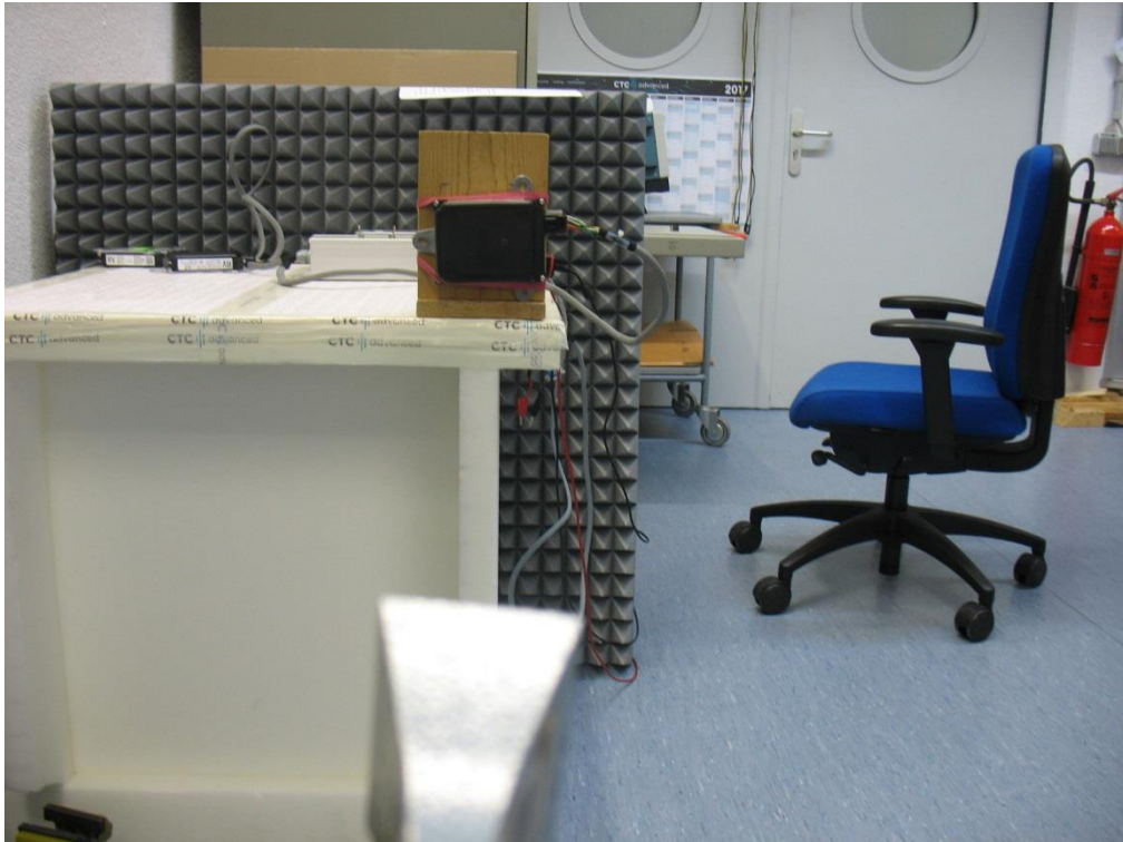
Photo 5: RSE set-up 18 GHz to 110 GHz, low / mid / high frequency
