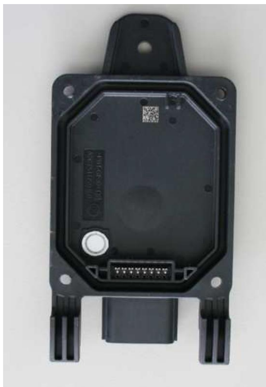
Photo 8: Housing inside - backcover
