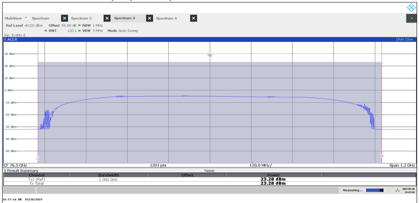
Plot 3: Radiated Mean Power (EIRP), Channel power, EUT1, Mode 17
