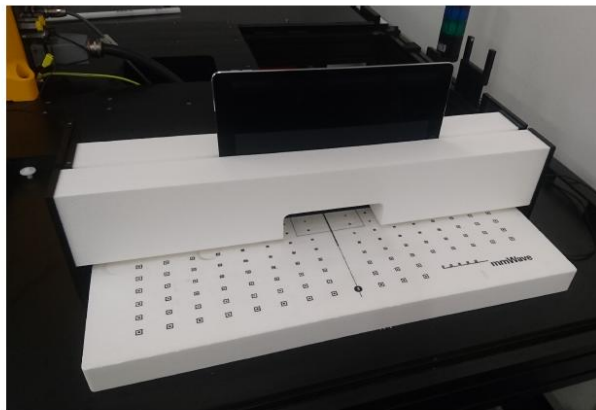
Figure 3.13.1: Test Setup with the mmWave Device Holder
