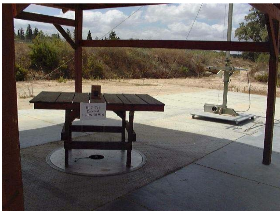
Figure 1. Radiated Emission Test 9kHz-30MHz
