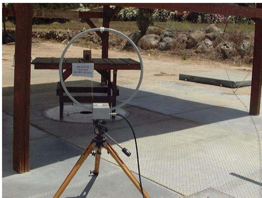
Figure 1. Radiated Emission Test 9kHz-30MHz
