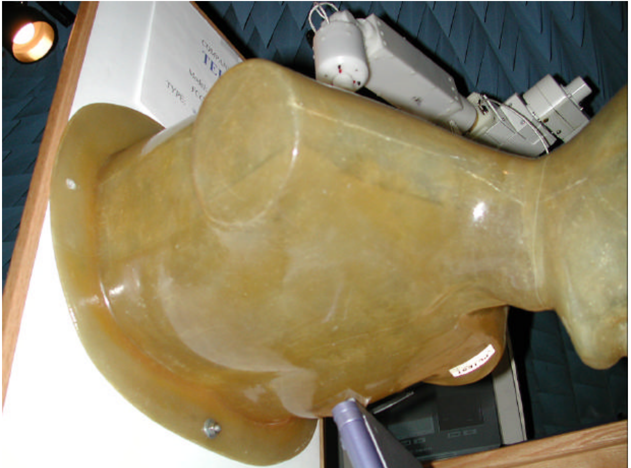
Figure 8. Test Setup of EUT in operating position with the source of significant emissions (antenna) 0.6 cm below the phantom.
