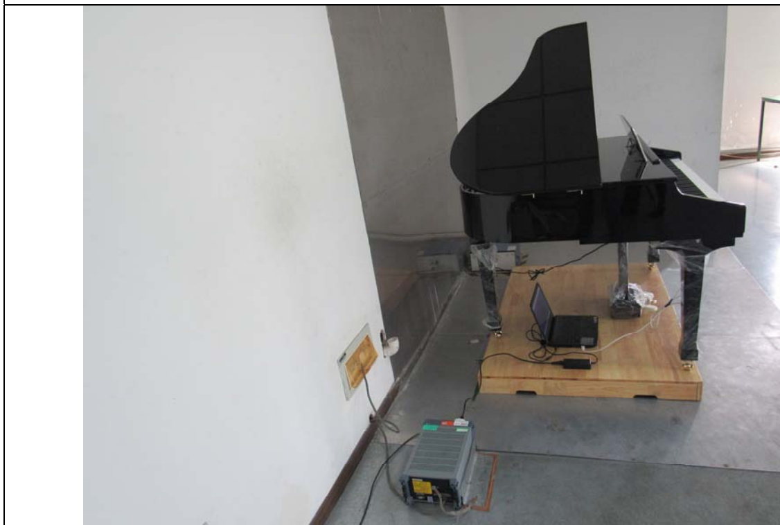
Conducted Emissions Setup Side View
