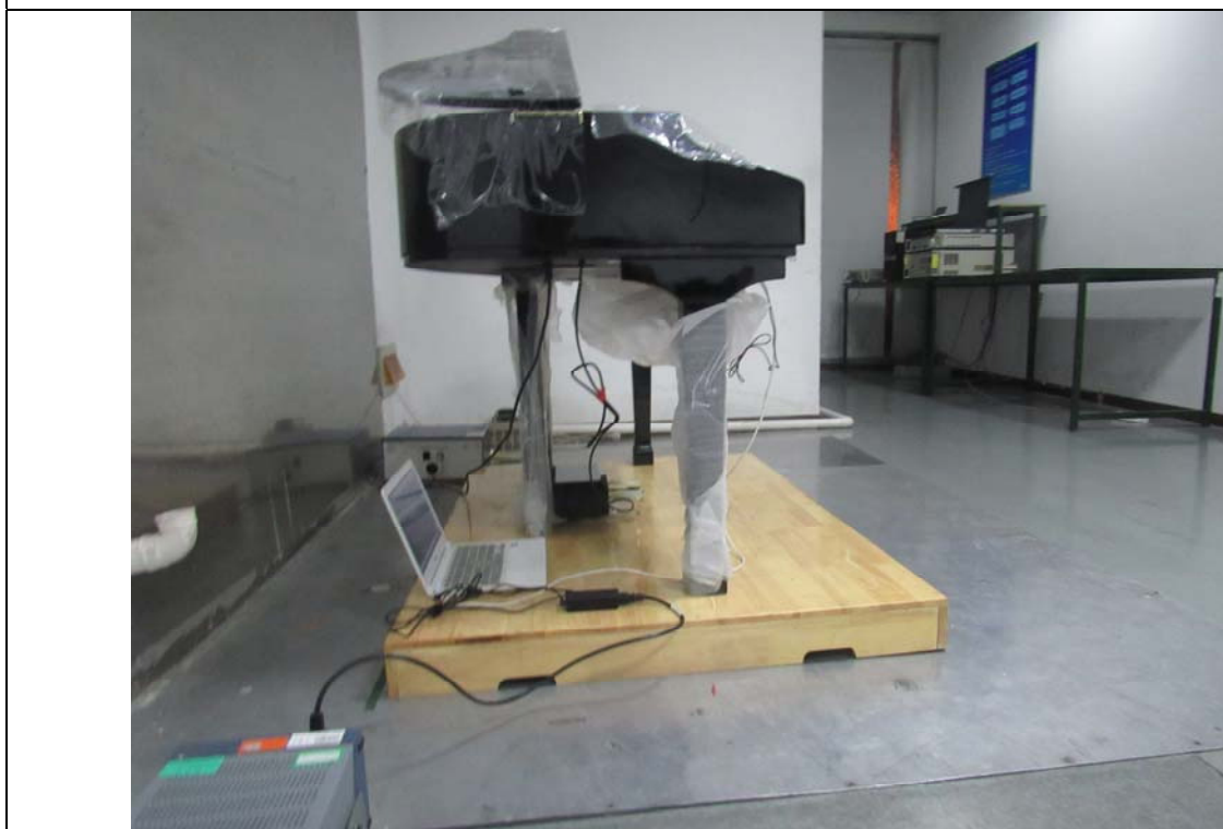
Conducted Emissions Setup Side View
