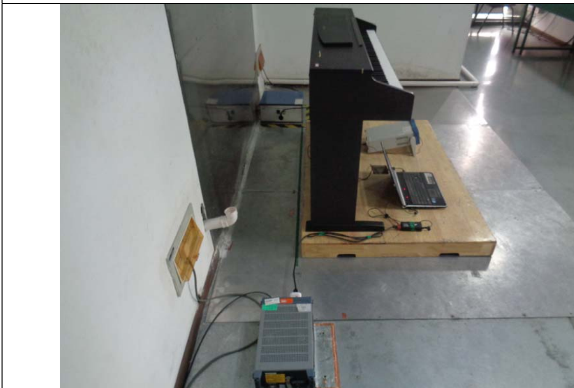
Conducted Emissions Setup Side View
