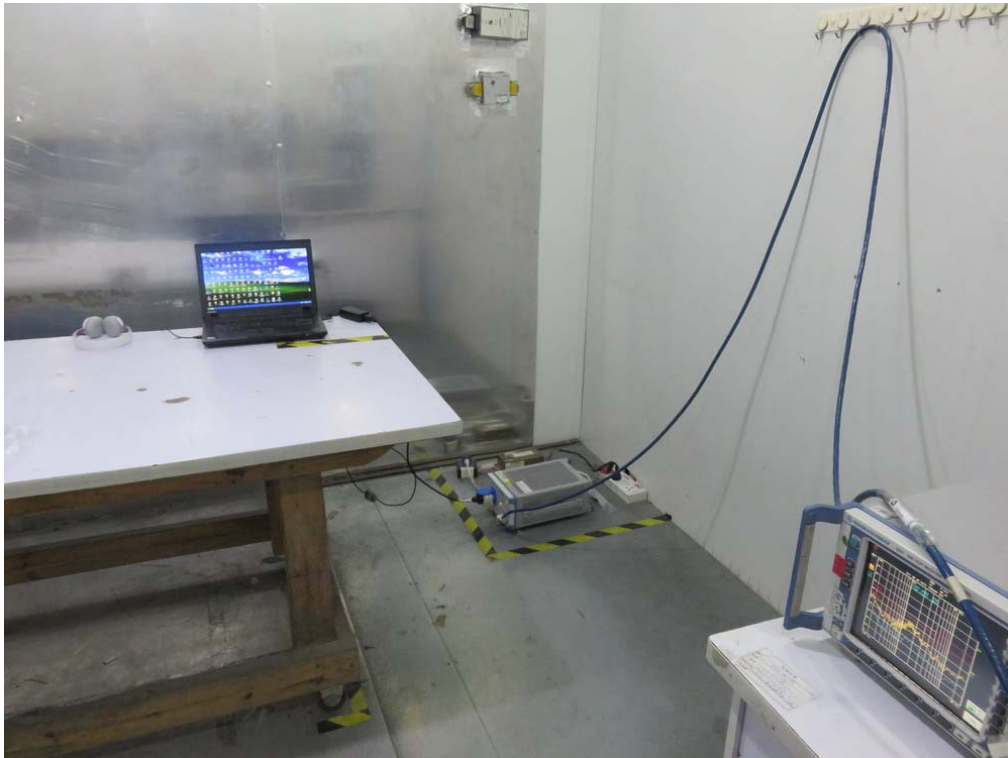
FCC RADIATED EMISSION TEST SETUP
