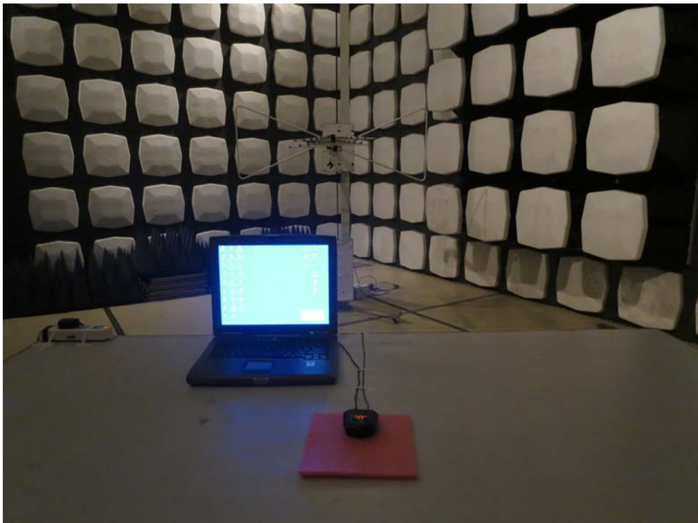
FCC RADIATED EMISSION TEST SETUP
