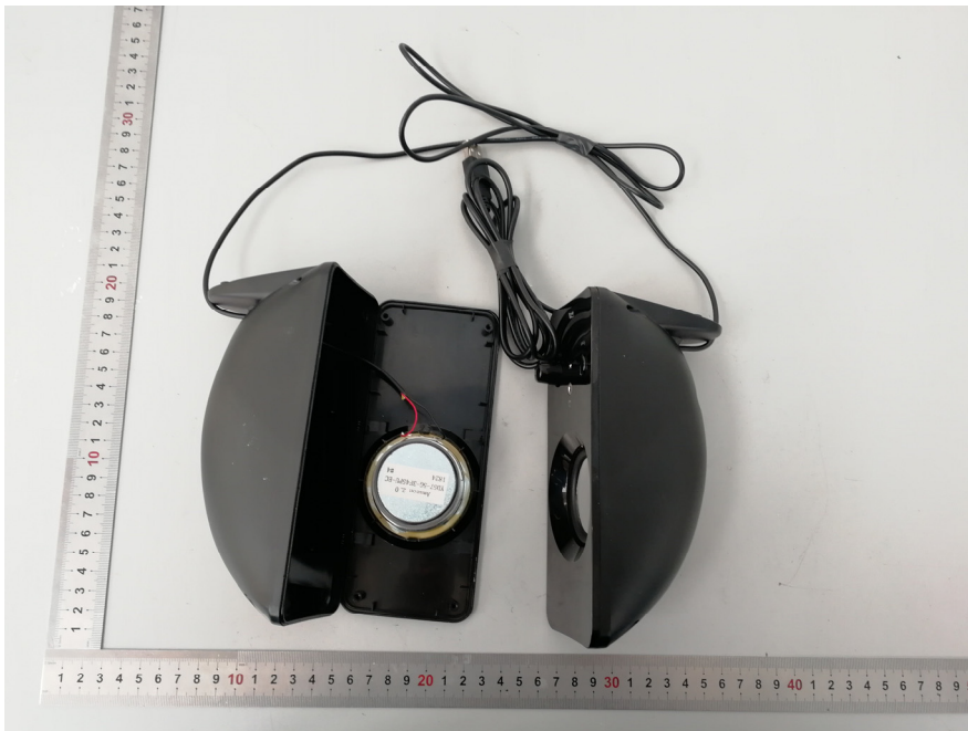
EUT – Cover off View-2
