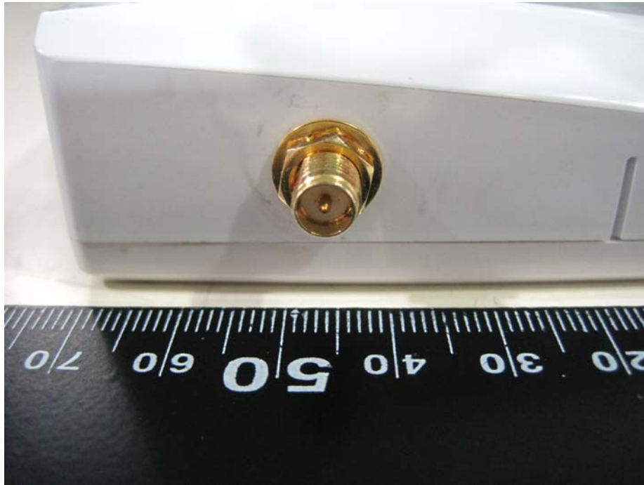
View of the Antenna Port
