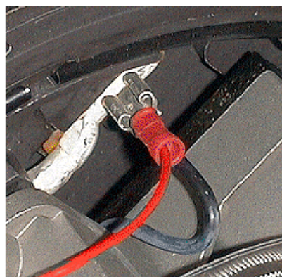
Insulated crimp connector option
