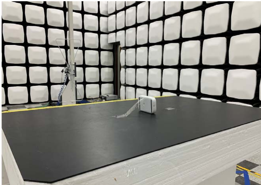
Radiated Test Picture(Rear)_Below 1GHz
