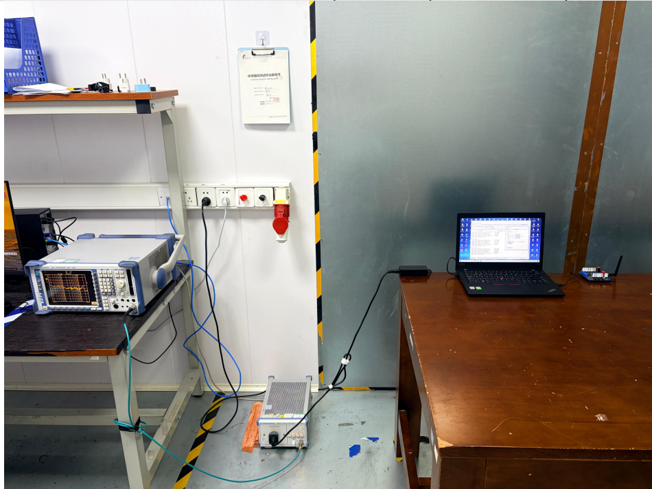
Conducted emissions at AC power line (150kHz-30MHz)
