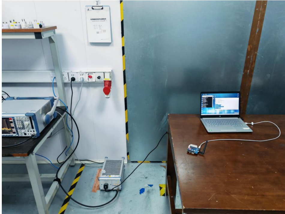
Conducted Emissions at Mains Terminals (150 kHz-30MHz)
