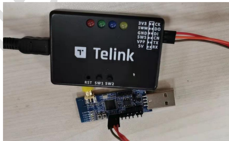
Figure 2-2 3.3V power supply
