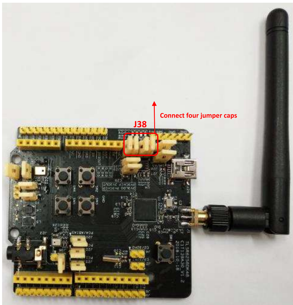
Figure 9 Connection chart to use PWM function
