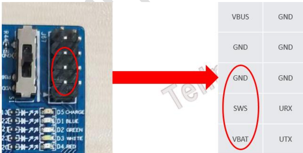
Figure 2-2 3.3V power supply
