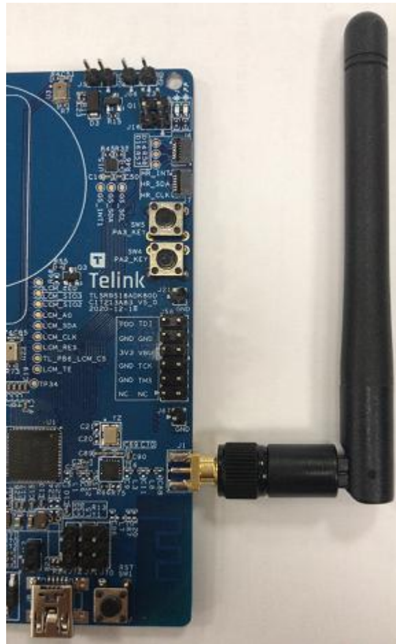
Figure 3-2 Chose 2.4G glue stick antenna
