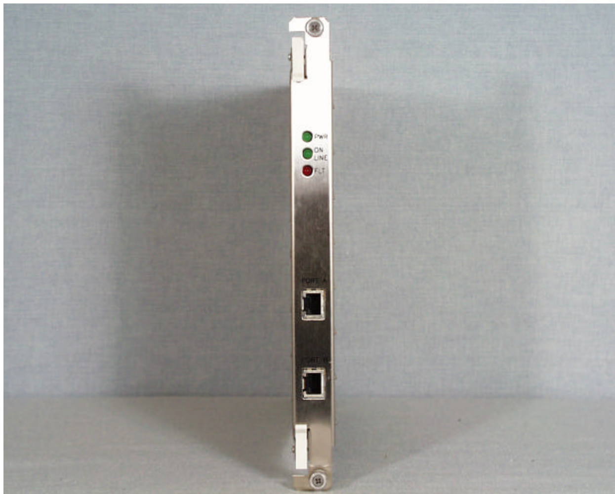
Front view of the 340122 2-port E1/T1 Interface board
