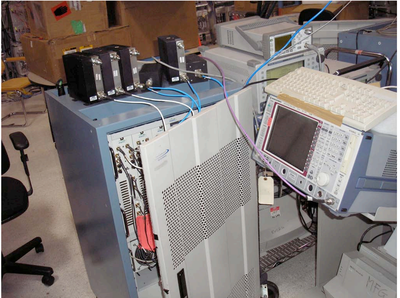
Antenna Port Conducted
