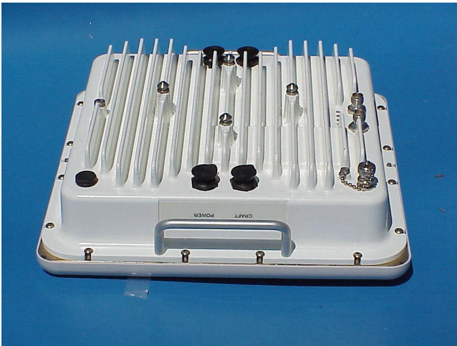
Link CX external side view showing power and craft connectors
