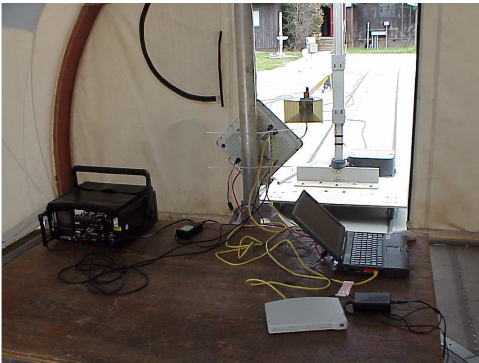
Link CX, 15.205 Radiated emissions, Restricted bands, setup
