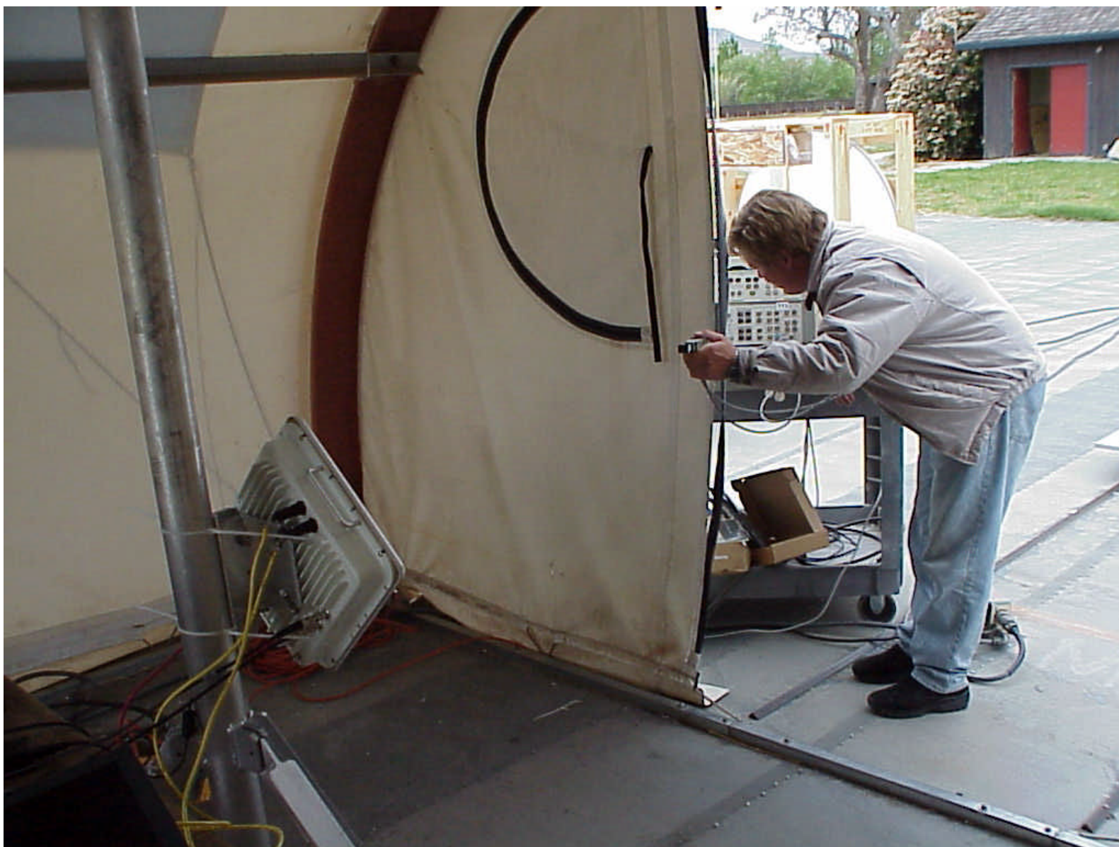
Link CX, 15.205 Radiated emissions, Restricted bands, setup
