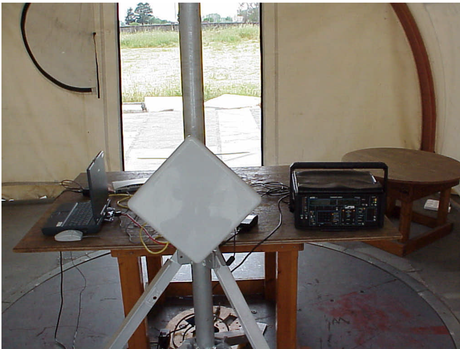
Link CX, 15.205 Radiated emissions, Restricted bands, setup
