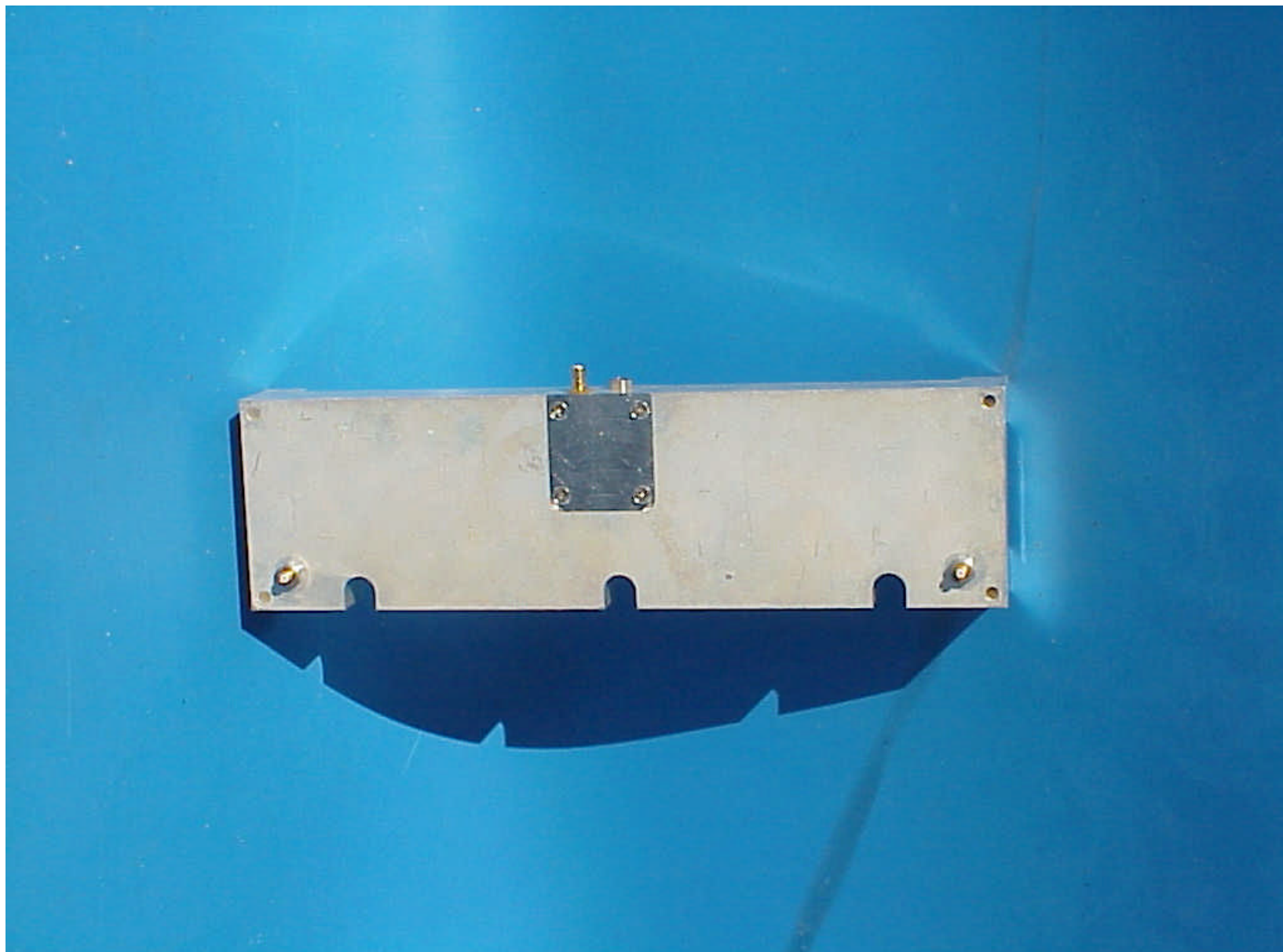
Link CX duplexer, bottom view
