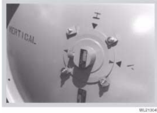
Figure 4-27 Feed Horn Installation for Vertical Polarized Operation
