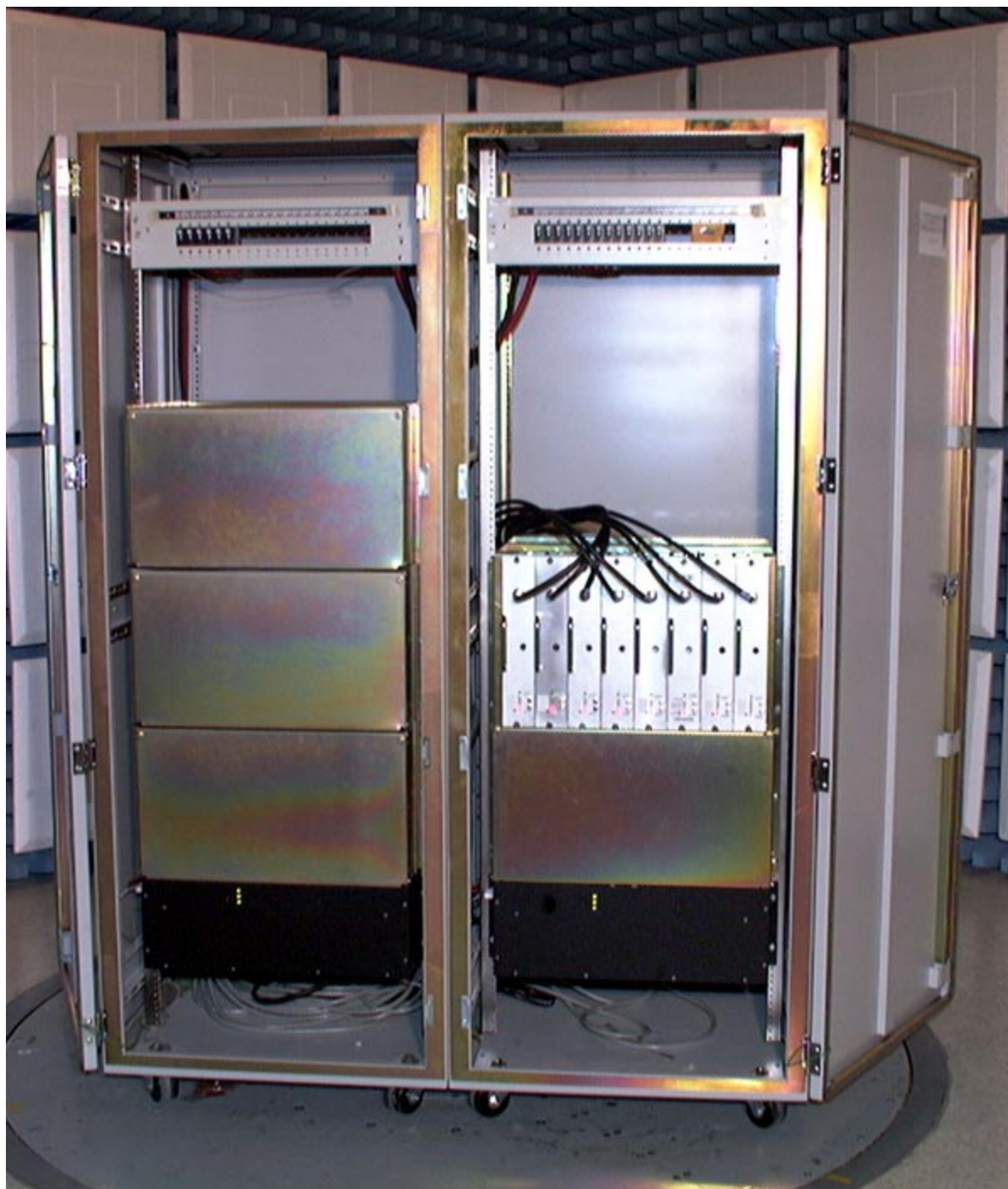
Figure 4.3 Front view of PWAN Base Cabinet - doors open
