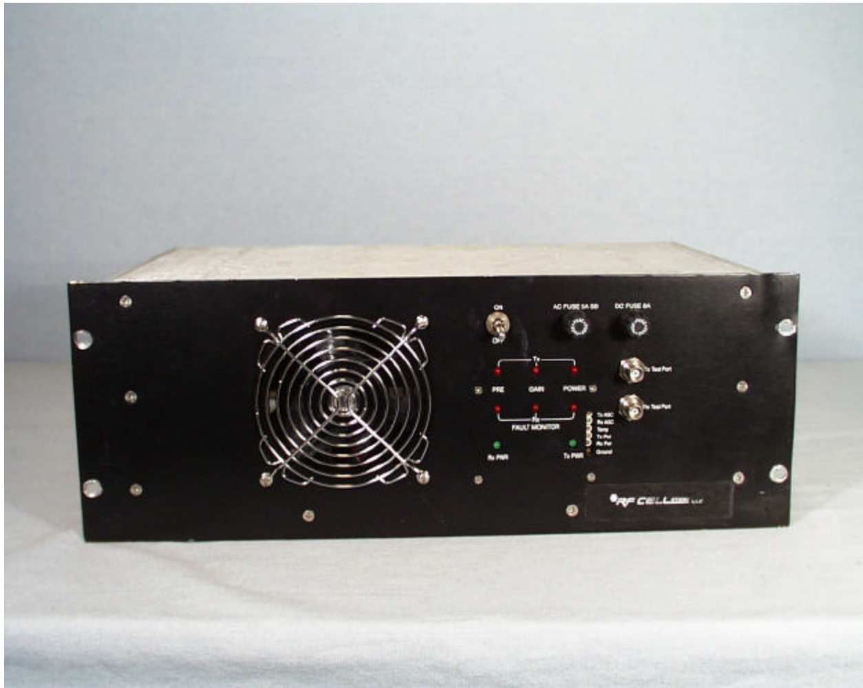
Front View of the Celwave BDA
