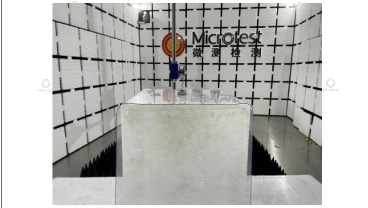
Radiated emission – above 1GHz
