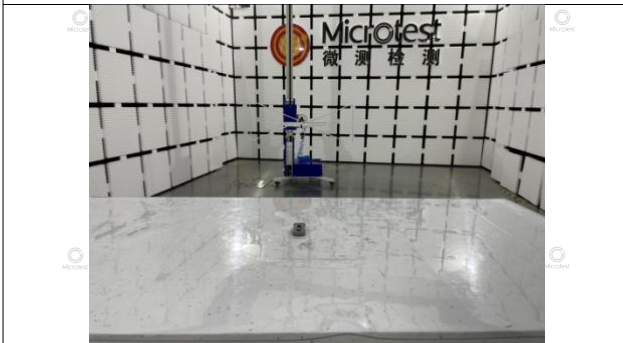
Radiated emission – above 1GHz
