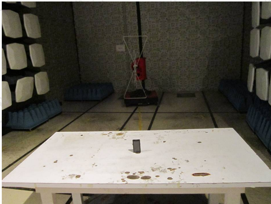
TEST SETUP OF RADIATED EMISSION (30MHz~1GHz)
