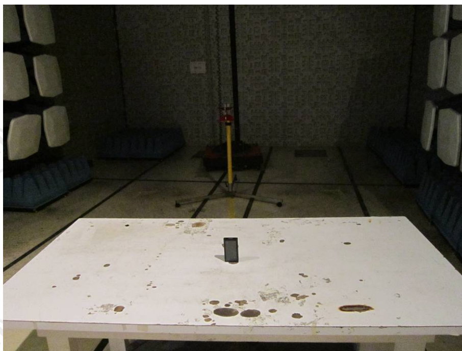
TEST SETUP OF RADIATED EMISSION (Above 1GHz)
