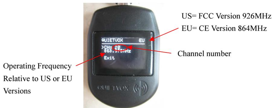
4) While the “>” cursor is pointing the Ch=xx, momentary press the [Volume Down] button to enter the channel selection as shown below:
