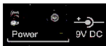
Picture 2.4. The power connector
