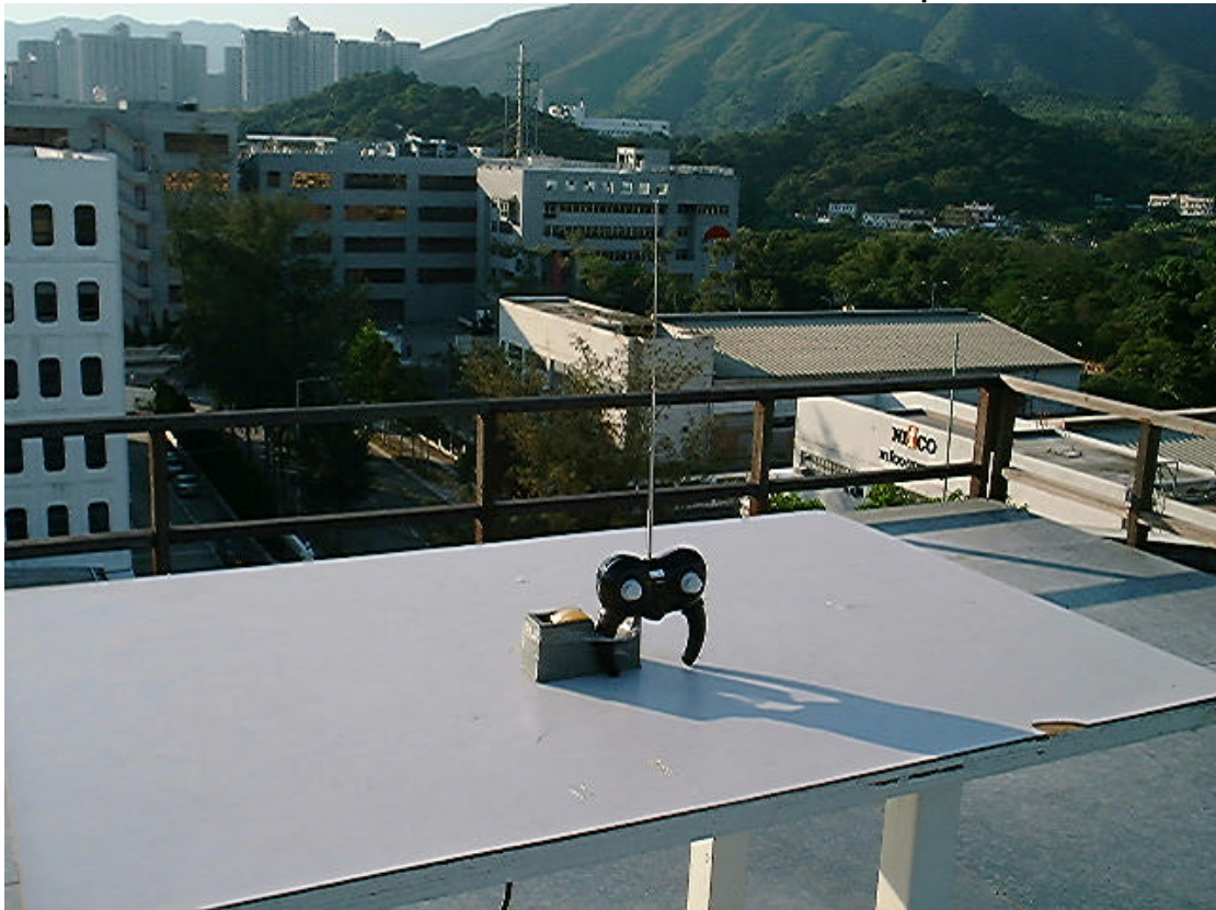
Measurement of Radiated Emission Test Set Up
