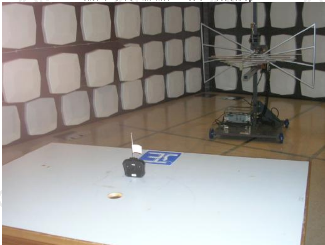
Measurement of Radiated Emission Test Set Up
