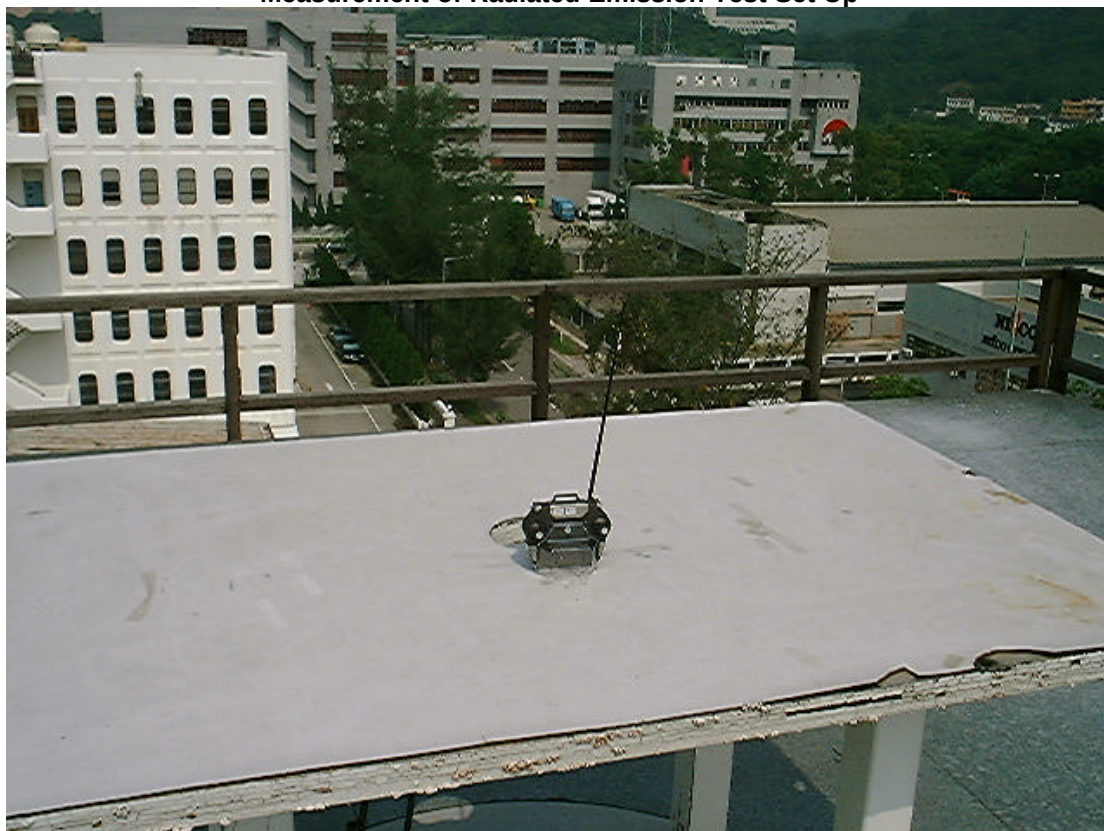
Measurement of Radiated Emission Test Set Up
