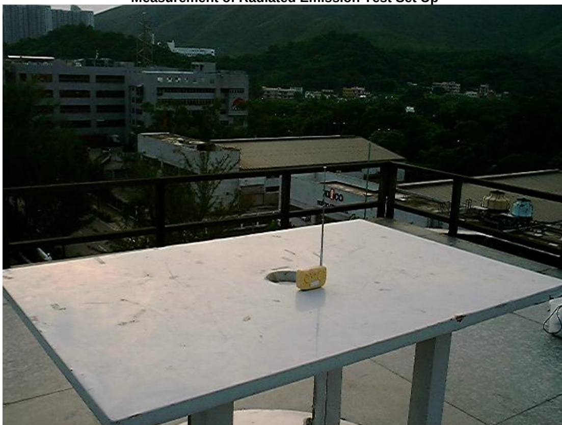
Measurement of Radiated Emission Test Set Up
