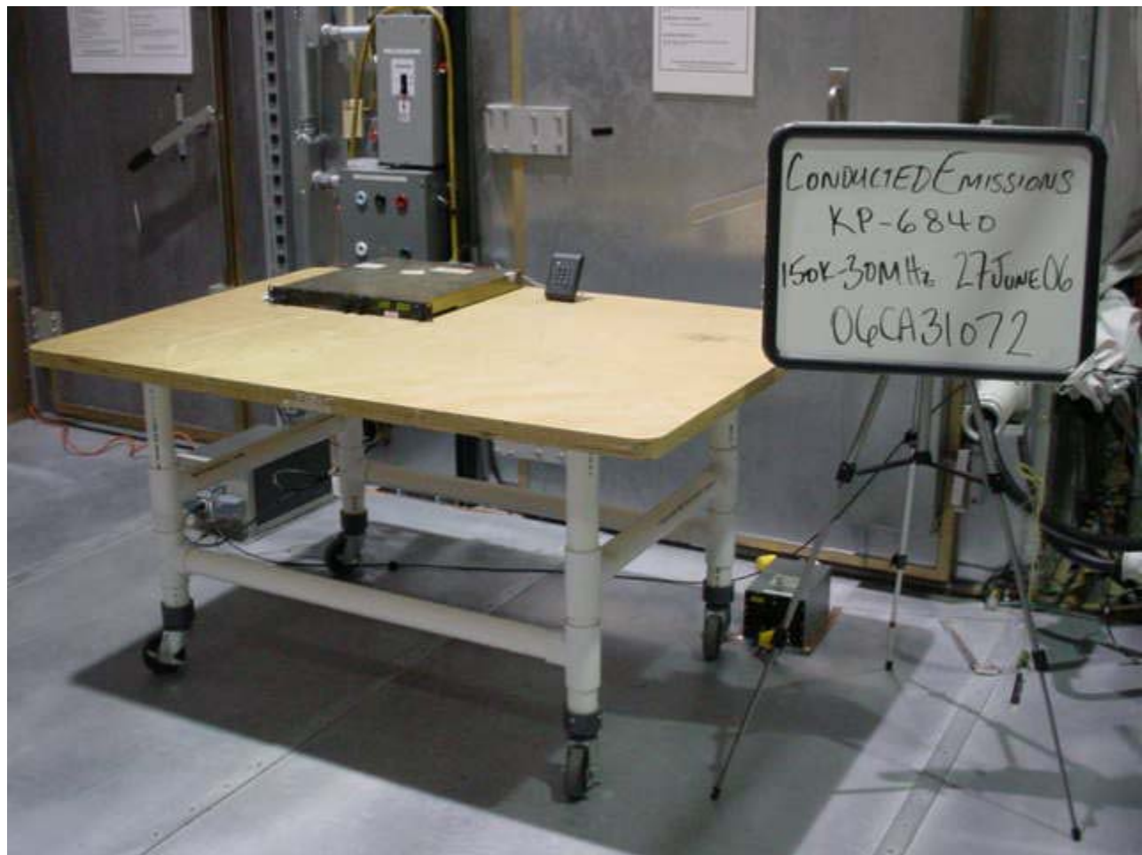
Conducted Emissions Test Setup (150kHz – 30MHz)
