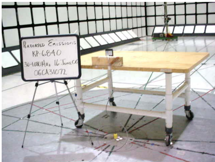
Radiated Emissions Test Setup (30 – 1000MHz)
