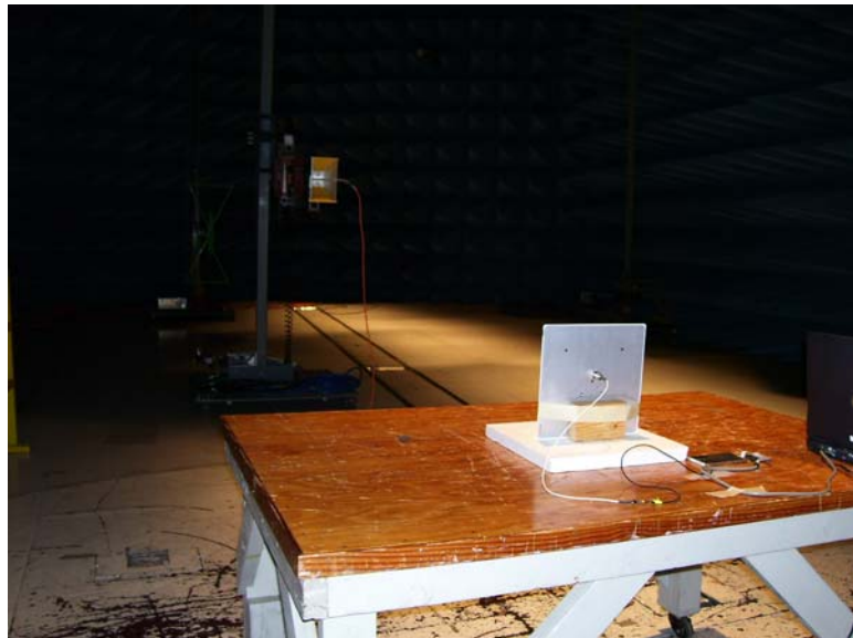
Photograph 9: Radiated measurements setup, Back View
