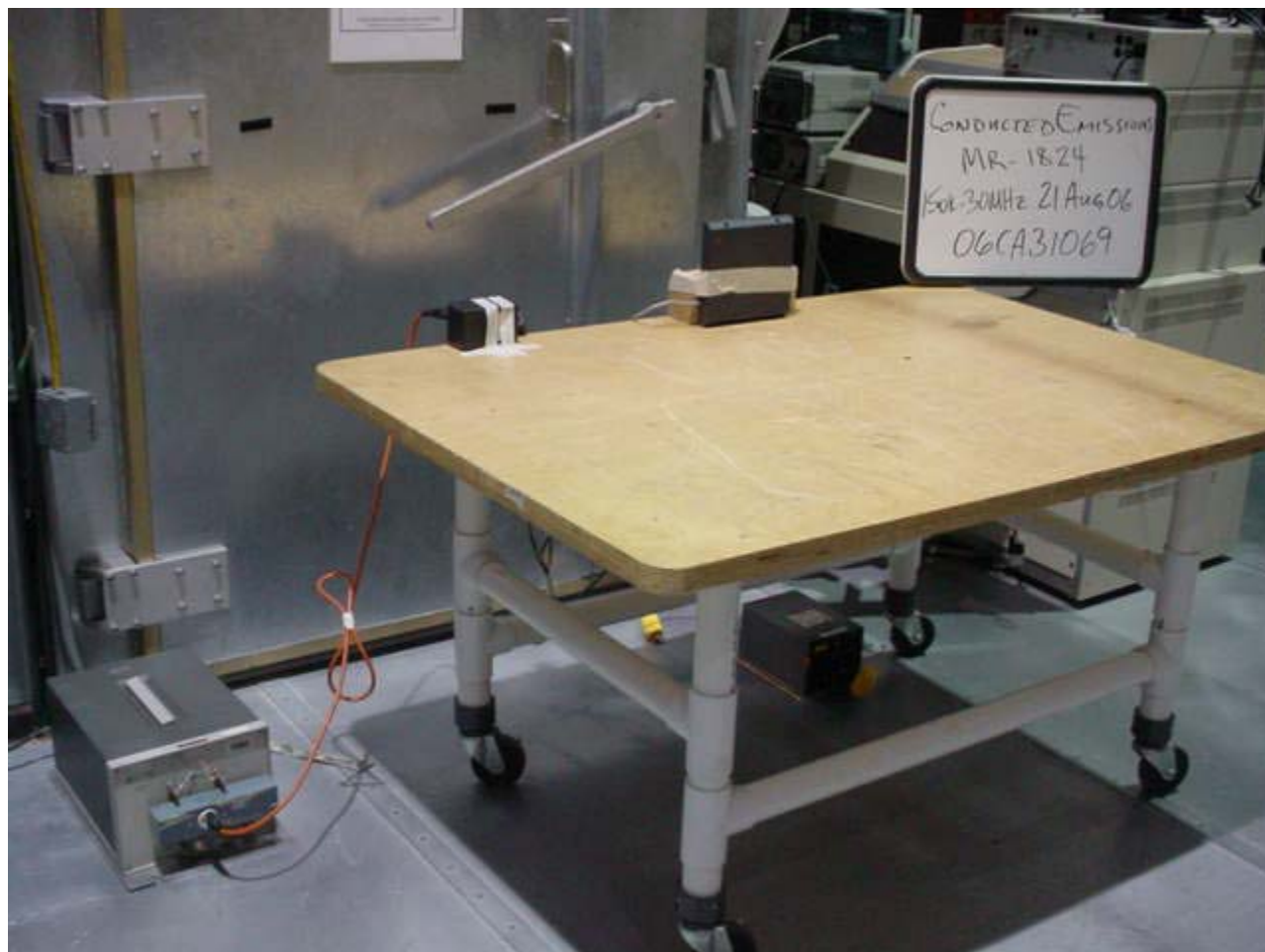
Conducted Emissions Test Setup (150kHz – 30MHz)
