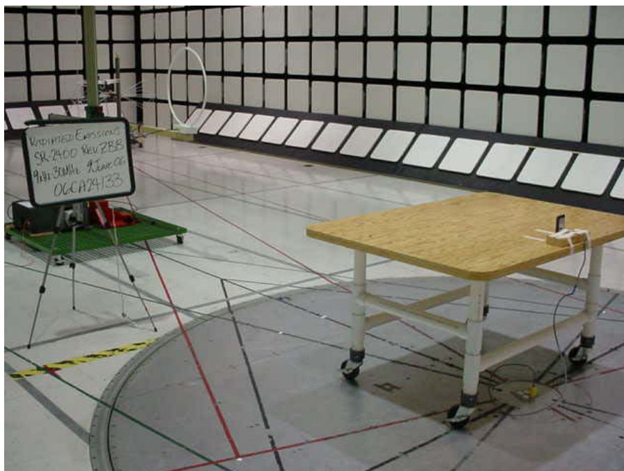
Radiated Emissions Test Setup (9kHz – 30MHz)
