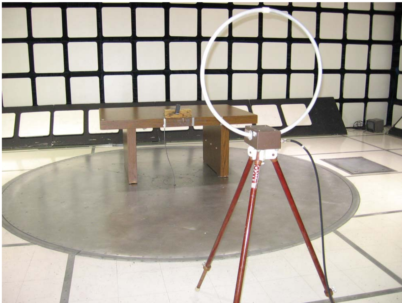
Radiated Emissions Test Setup (9kHz – 30MHz)
