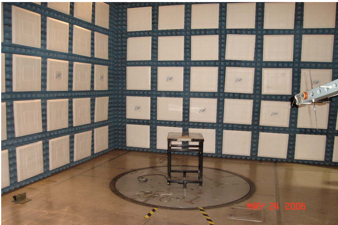
Test Set-up for Radiated Emissions Vertical Polarity
