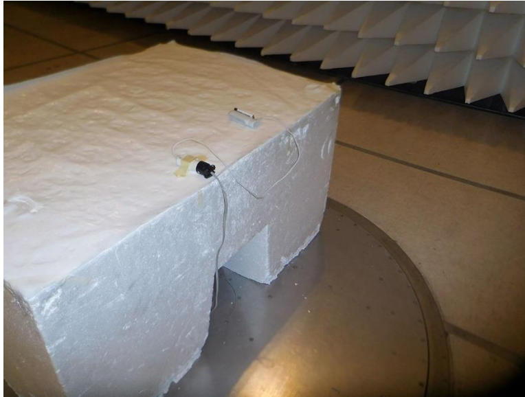
Charger with Load, Below 1GHz, 0.8m
