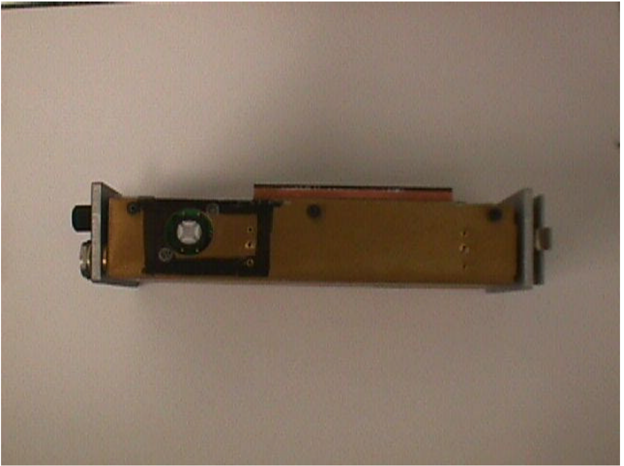
D15: SIDE VIEW OF TX SWITCH ON/OFF
