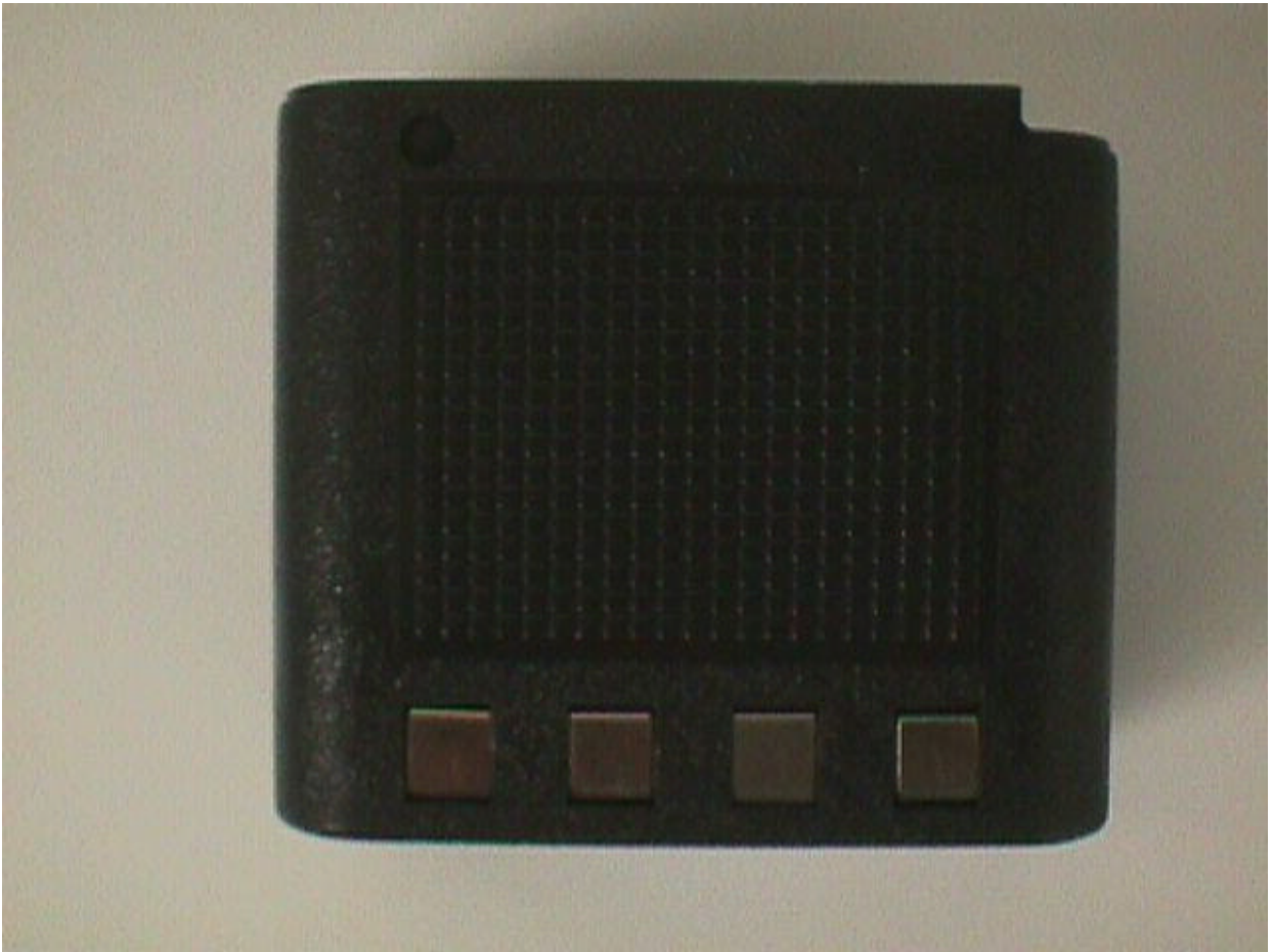
D27: BATTERY CONNECTIONS FOR EXTERNAL CHARGER
