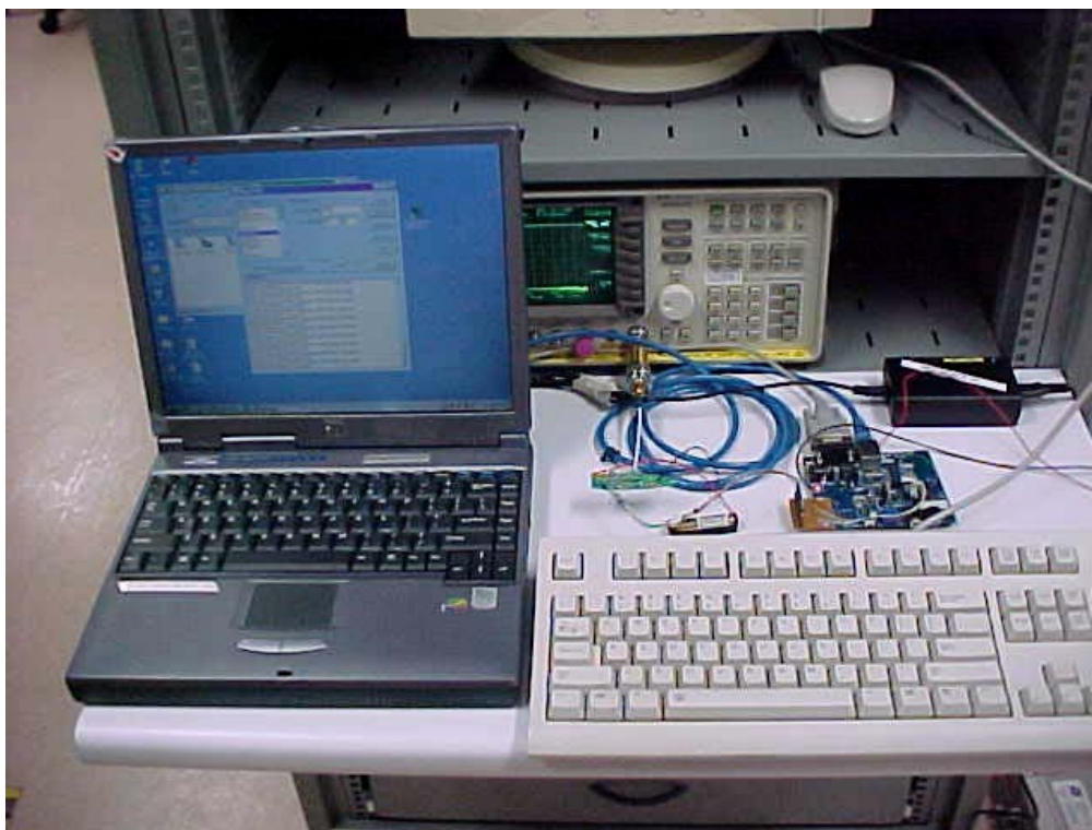
Number of Hopping Frequencies Measurement Test Setup
