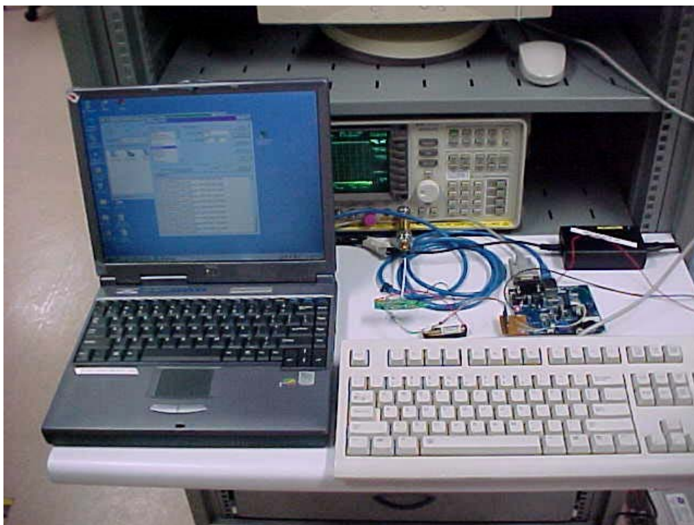
Spectrum Bandwidth Measurement Test Setup
