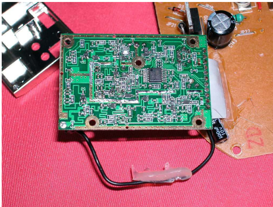
Base Oscillator PCB solder side
