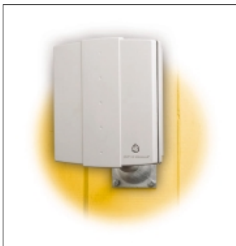
Figure 7-6 Outdoor Subscriber Unit Mounted on Wall
